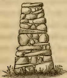
A SECTION OF WALL WELL LAID.
