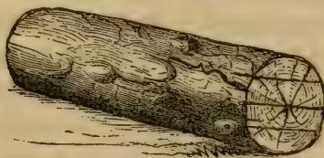
MANNER OF SPLITTING A LOG INTO FOUR POSTS.
