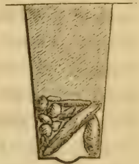
STONING WITH ONE ROW OF SIDE STONES.
