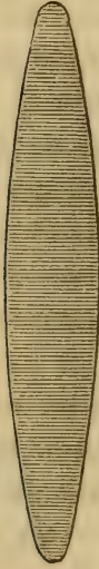
A TRANSVERSE SECTION OF THE BLADE OR BIT OF A WELL-FORMED CHOPPING AXE.
