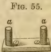
FIG. 55. INSTRUMENT FOR BENDING THE WIRE.
